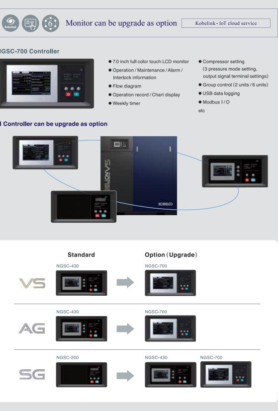
Energy saving logic USB data logging Modbus I / O
