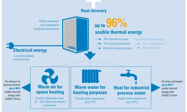
\*The ALMiG F-Drive not only uses energy from the oil cooling circuit, but thanks to the oil cooling of the electric motor this energy can also be recovered.
