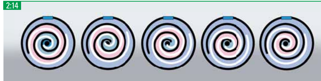
Compression principle of a scroll compressor.
