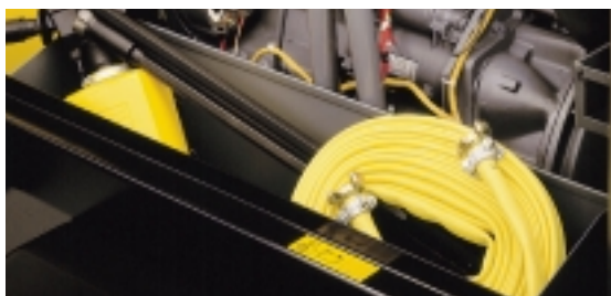
Pneumatic equipment such as hoses and breakers can easily be locked away inside the canopy if no generator is installed.
