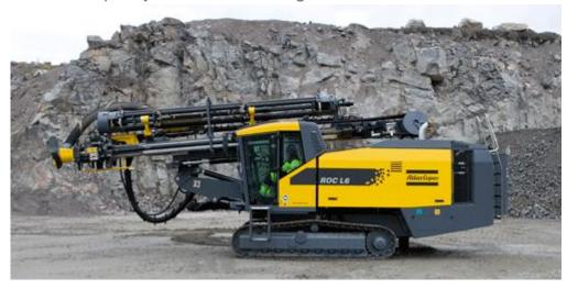
ROC L6(25) and L6(30) are high-capacity down-the-hole crawlers for quarry drilling in soft, medium and hard rock, with Atlas Copco screw type high pressure compressors that delivers compressed air at full 25 and 30 bar. With the powerful CAT C11 and CAT C13 diesel engines the ROC L6 not only provides power, but economy.
