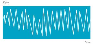
The ZH 350<sup>+</sup> handles air demand fluctuations more effectively than turbo technology could do up to now. Its fast transitions between load and unload operation eliminate the need for expensive blow-down of compressed air in times of low air demand.
