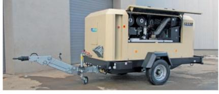
The wide opening doors and standard central drains contribute to the excellent serviceability of the 12/150, with all areas carefully designed for ease of inspection, maintenance and repair.
