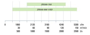
ZT: Air cooled / ZR: Water cooled / VSD: Variable Speed Drive See data pages for range details
