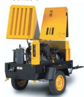
The canopy doors open diagonally with the help of pneumatic springs to give you easy access to the machinery. With the doors up and out of the way, you can perform routine maintenance in less time.
