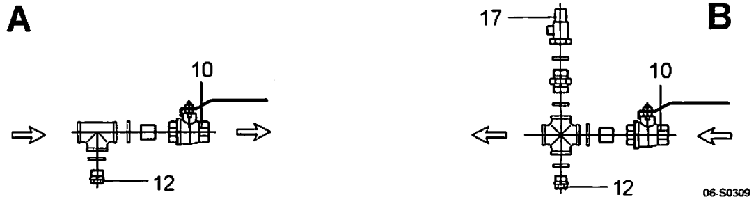
Fig. 14 Connecting the cooling water
