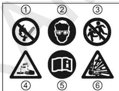
Fig. 51 Safety signs - warning stickers on the battery.
