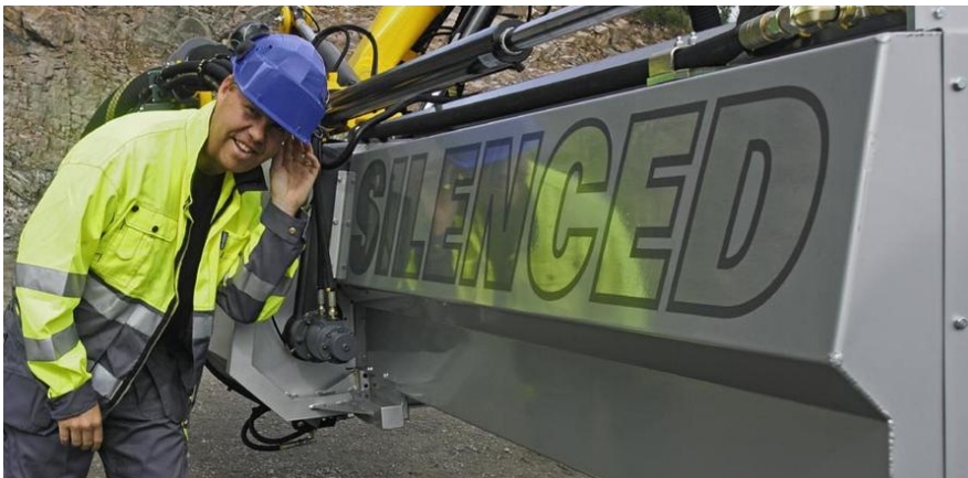
The optional Silencing Kit enables the SmartRig ROC D7C to be used in restricted urban areas.
