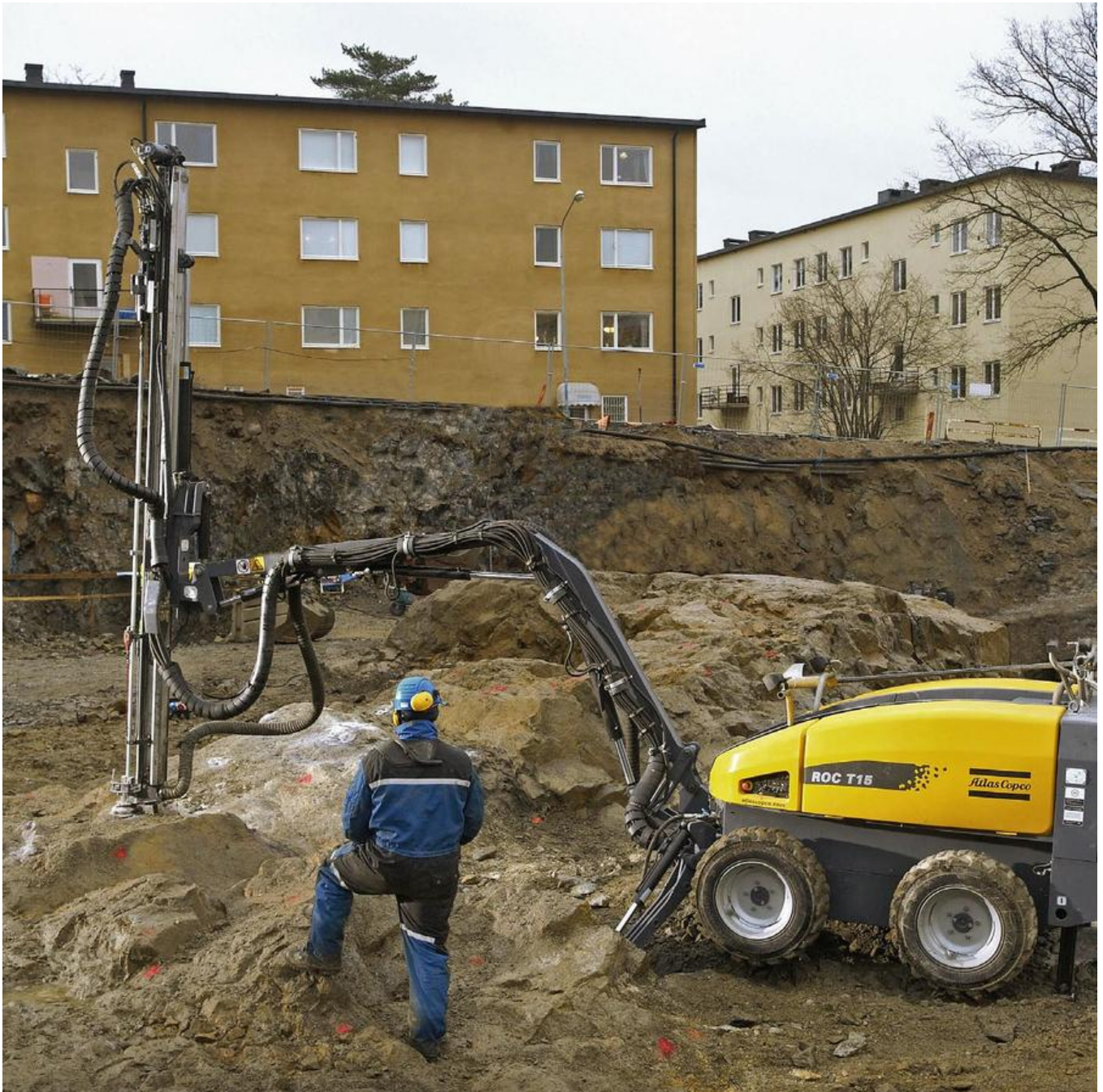
ROC T15 is a versatile and compact hydraulic drill rig for 22-45 mm diameter holes.
