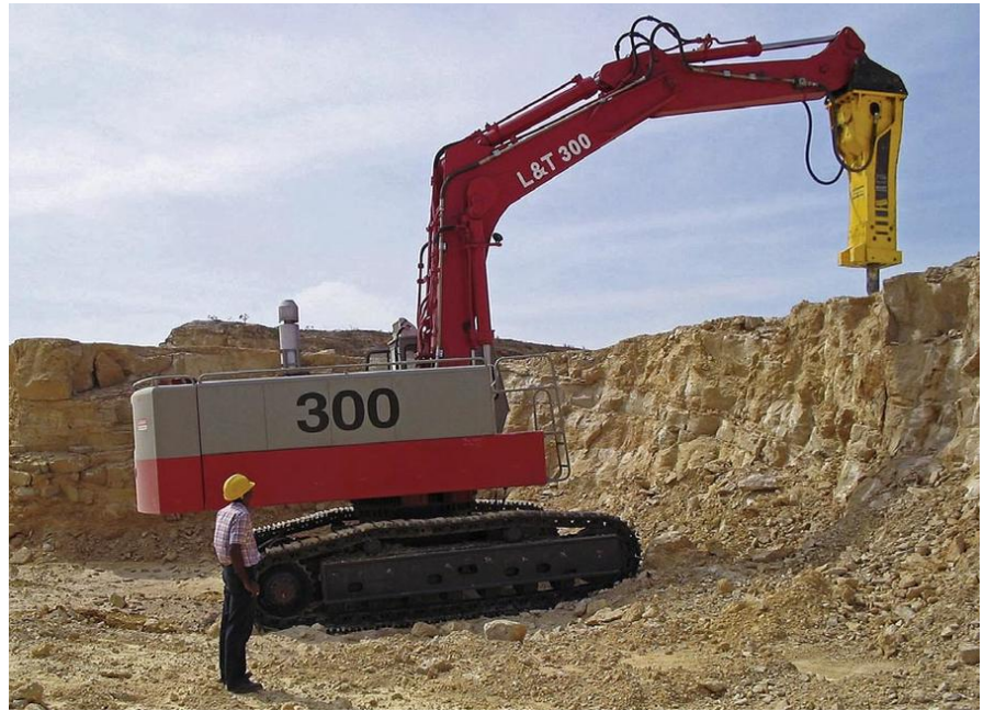
Hydraulic breaker HB 5800 attached to a 60 t excavator.
