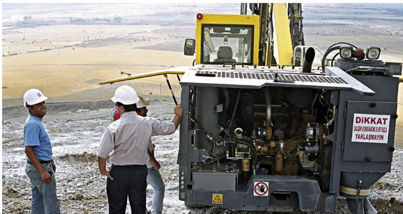
The larger canopy doors on the new ROC D7 rig enhance service access.
