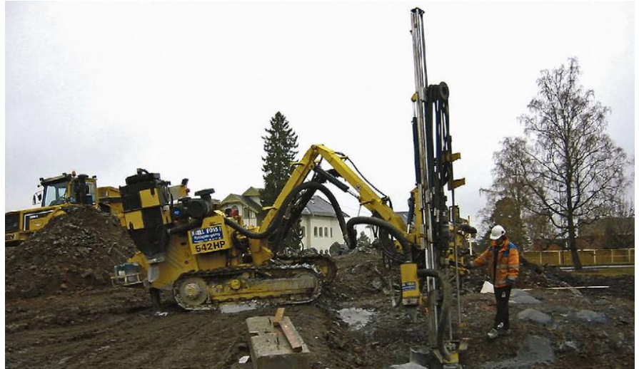
ROC 542HP repowered by COP 1640.
