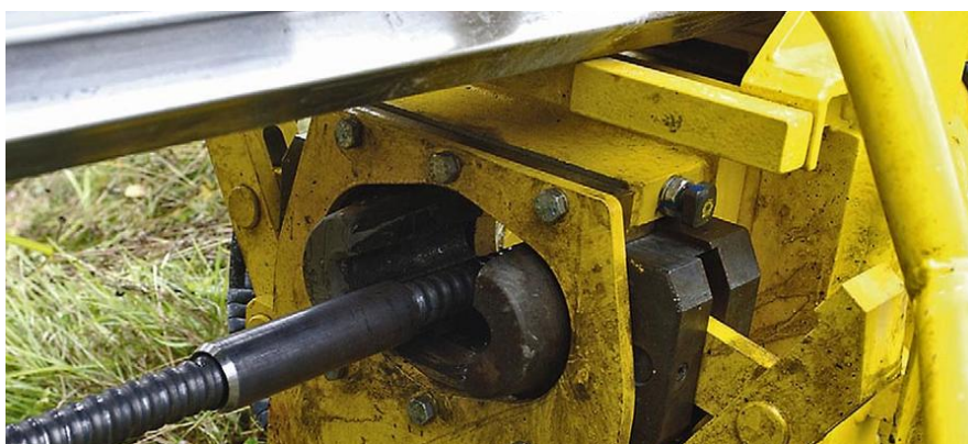
The special bushing halves prepared for firm gripping of the SDAs.
