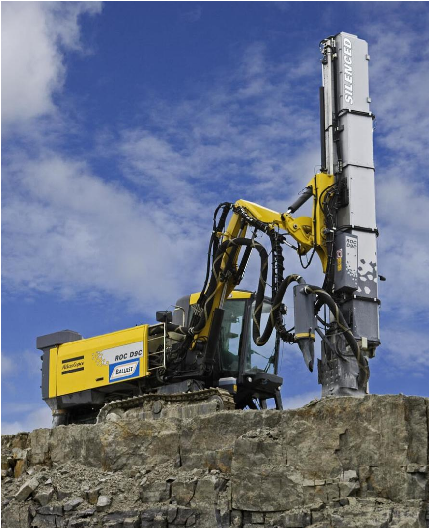
The SmartRig ROC D9C can be fitted with a unique silencing kit which reduces drilling noise to about 10 dB(A) below that of comparable rigs.
