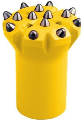
Secoroc full-ballistic button bit (dia. 127 mm) model –47–66. Flat front with same size front and gauge buttons.
