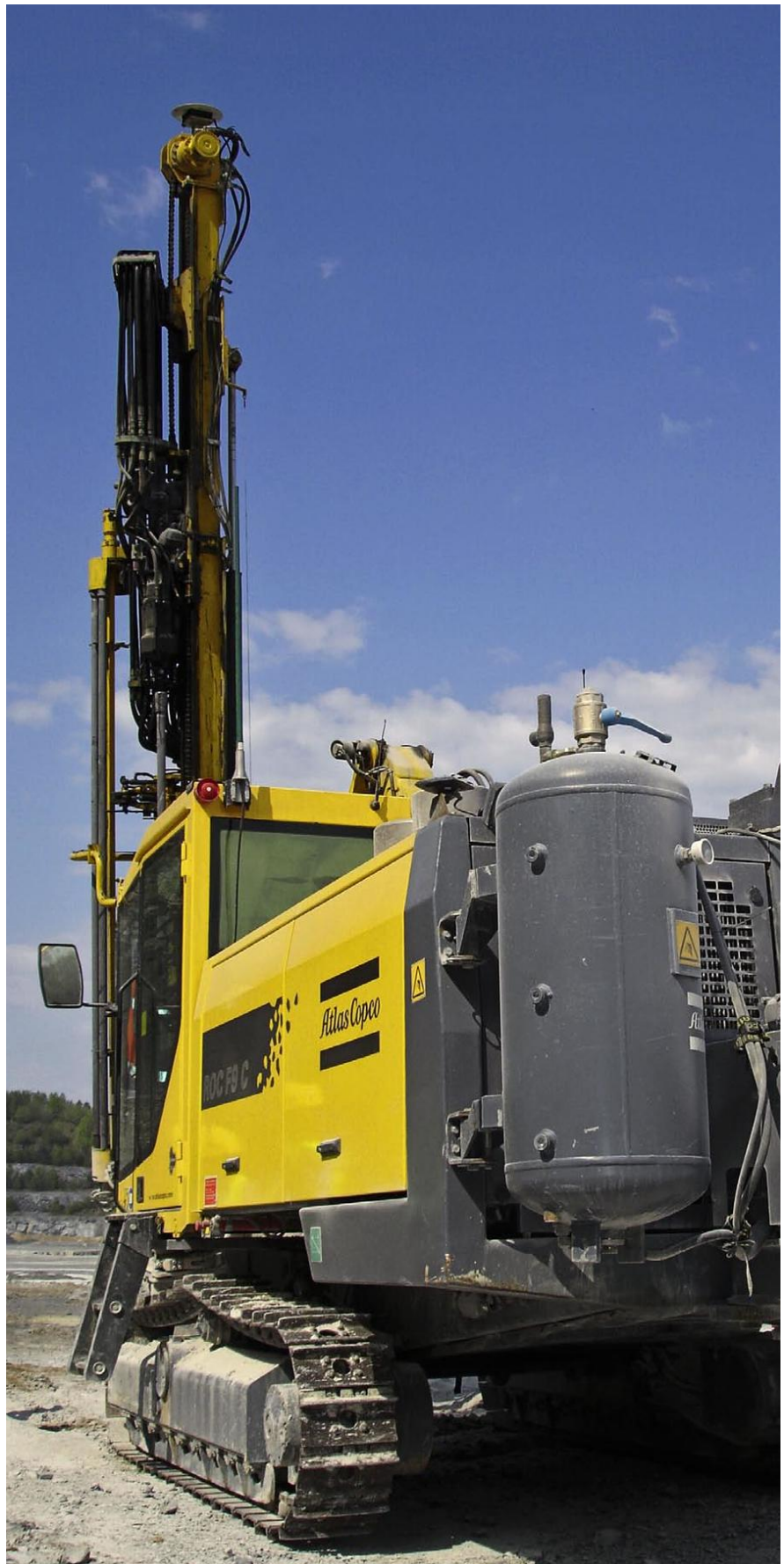
The HNS system on the SmartRig ROC F9C helps with positioning and performance monitoring.
