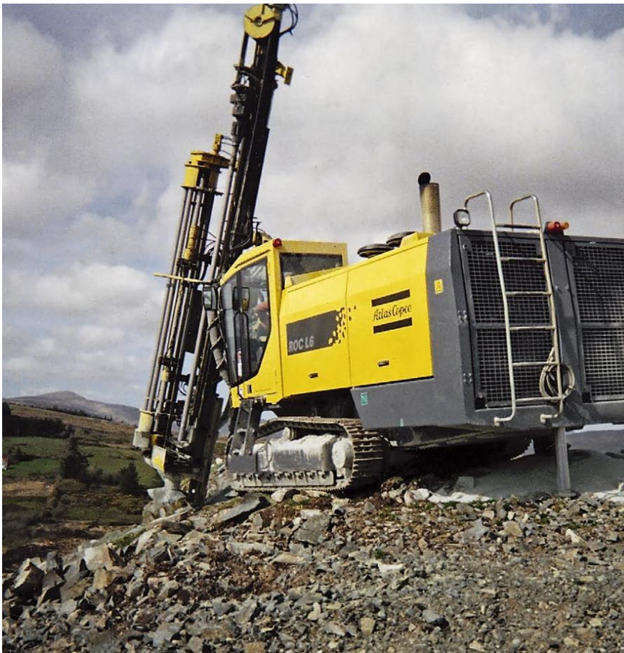
ROC L6 drilling in whinstone at Churchill Quarry, Donegal prior to addition of water tank.
