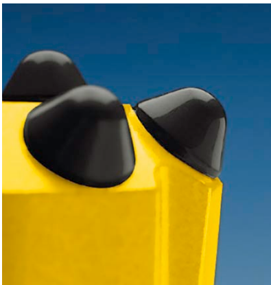
The full-ballistic buttons protrude more from the bit body, resulting in faster penetration in soft rock.
