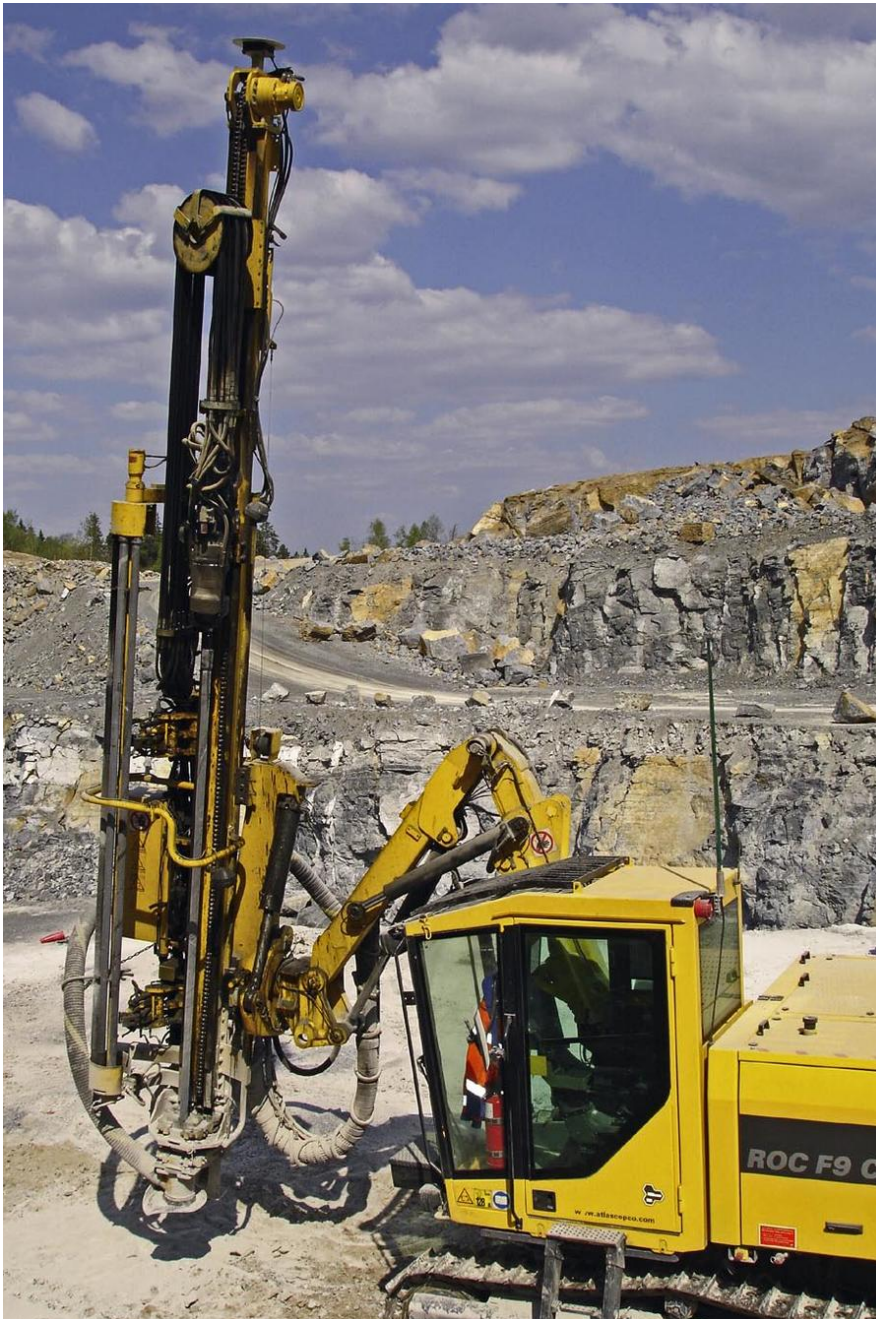
Statistics from the Bjørntvet quarry show a 25% reduction in use of explosives and a 40% drop in secondary blasting with SmartRig.
