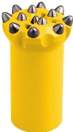
Secoroc full-ballistic button bit (dia. 76 mm) model –21–66. Drop centre front with larger gauge buttons.
