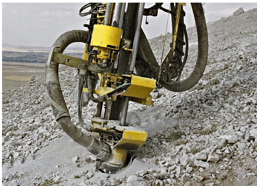
The stiffer square-section boom of the new ROC D7 aids more accurate collaring.
