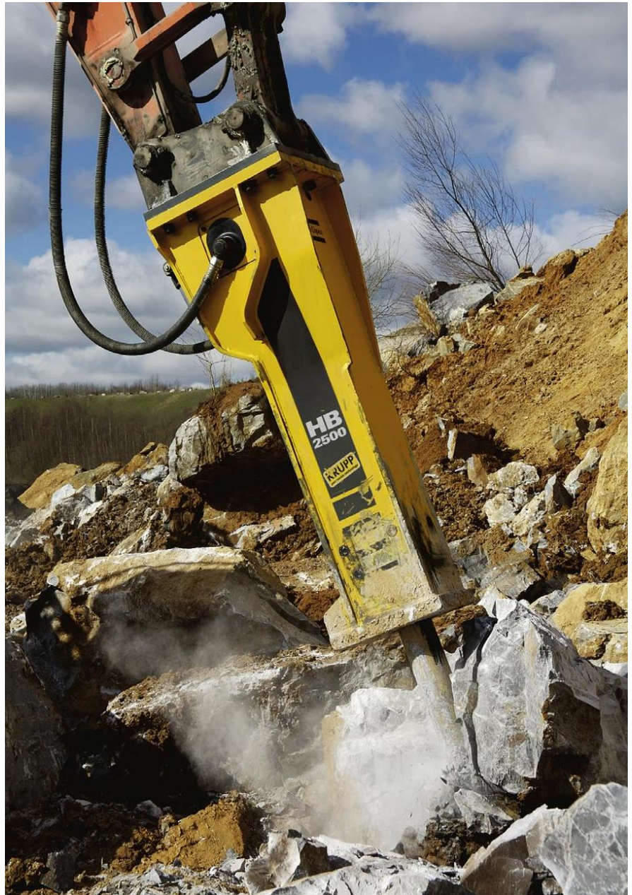
An HB 2500 used in secondary breaking.
