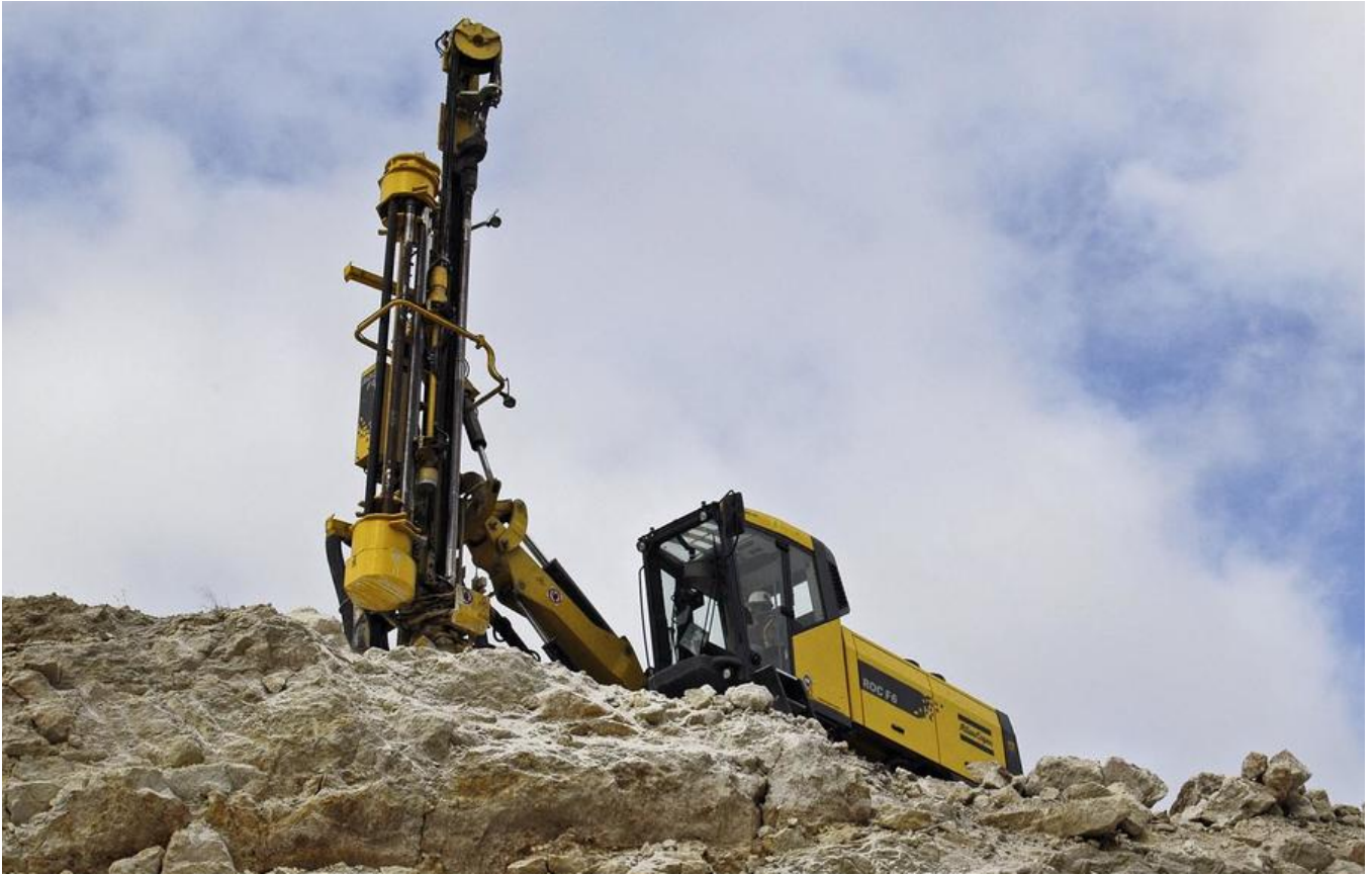
Atlas Copco ROC F6 achieves 3 m/min in soft limestone at Pinarhisar.
