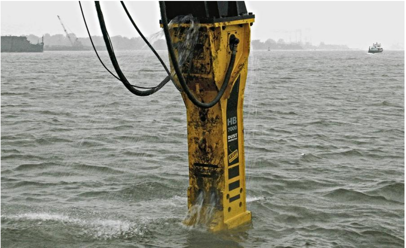
Atlas Copco HB 7000 with underwater kit.
