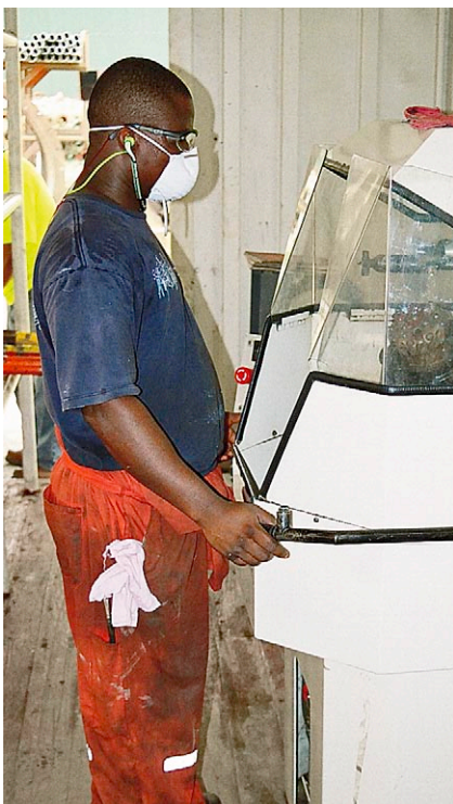
Professional bit grinding: training by Atlas Copco enabled Golden Star to set up its own bit grinding operations at the Bogoso/Prestea mines using the Secoroc Grind Matic machine.
