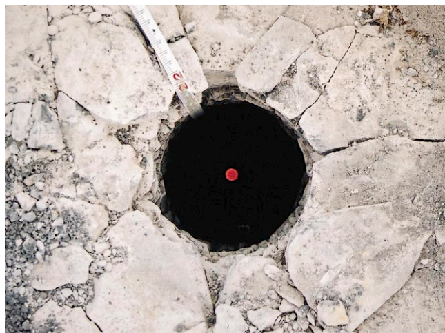
Perfectly straight vertical 22 m deep x 140 mm diameter hole drilled by the ROC L6 with COP 54 at Roadstone Quarry, Ballintra.
