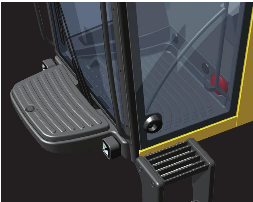
Stepping up: A service platform, which is also a toolbox, gives access to the windscreen; steps, grab rails and front mounted cab door make getting in and out easier; a single-moulded mat for easy cleaning.
