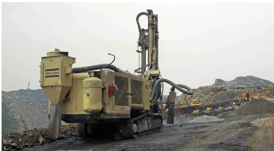
Drilling at Yingde Conch: an Atlas Copco CM 760 D surface crawler.
