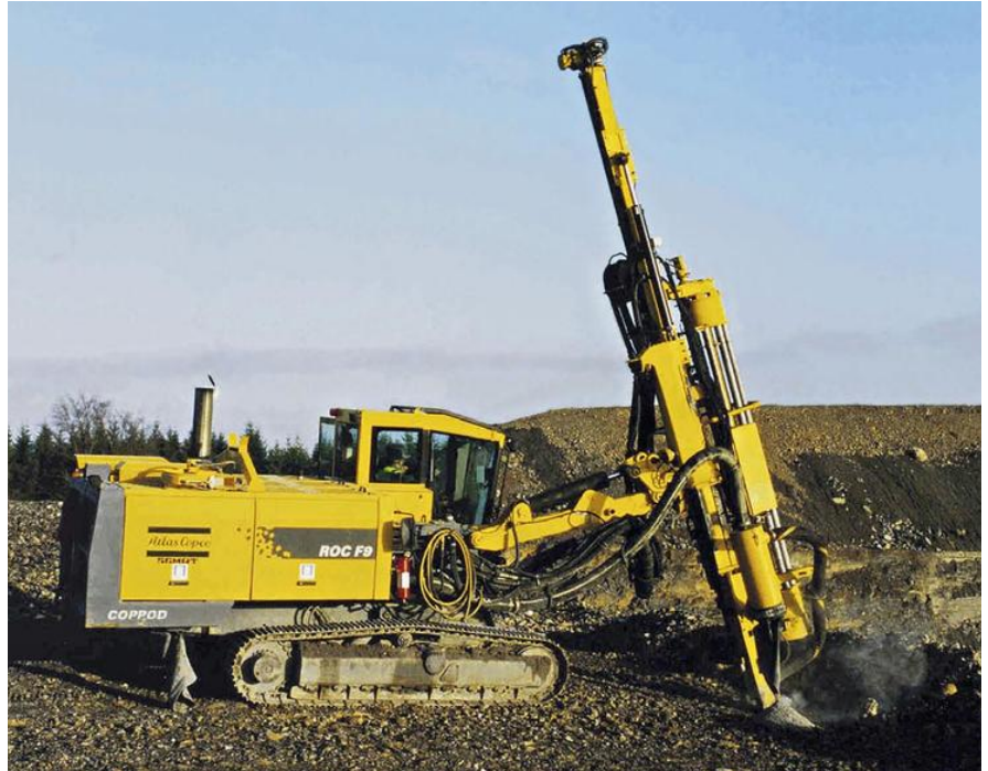
First in the fleet: the five-year-old ROC F9CR, now fitted with the second generation COPROD.
