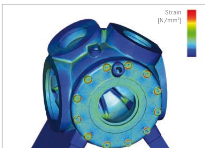
Top left: Piston Centre left: Honed cylinder interior Bottom left: FEM calculation for crankcase Right: BK 26 compressor block
