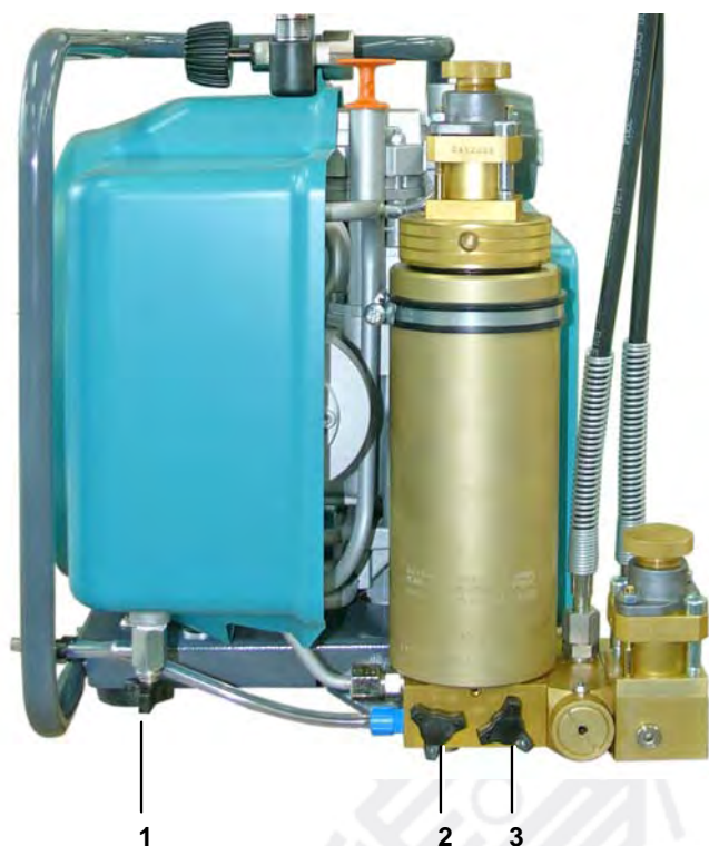
Abb. 28 Condensate drain taps
