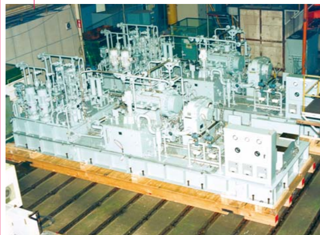
BCH303 Gas Turbine Fuel Booster Compressor
