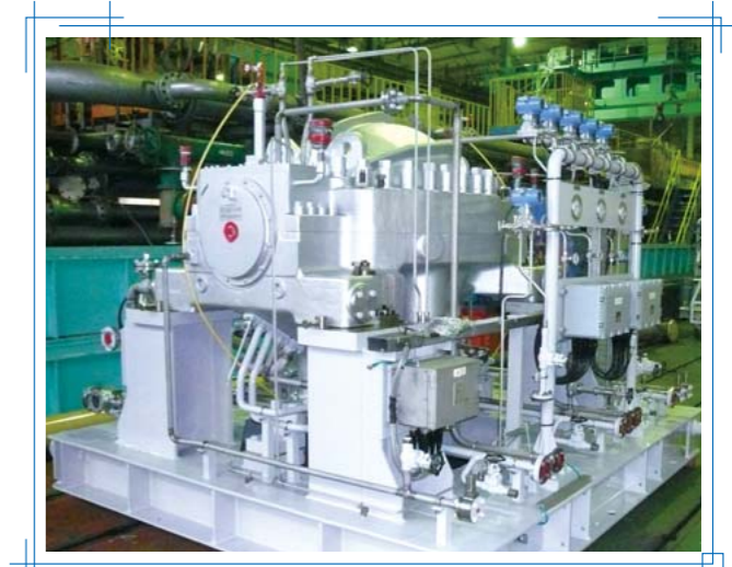
3MCH457 Ethylene Ref. Compressor
