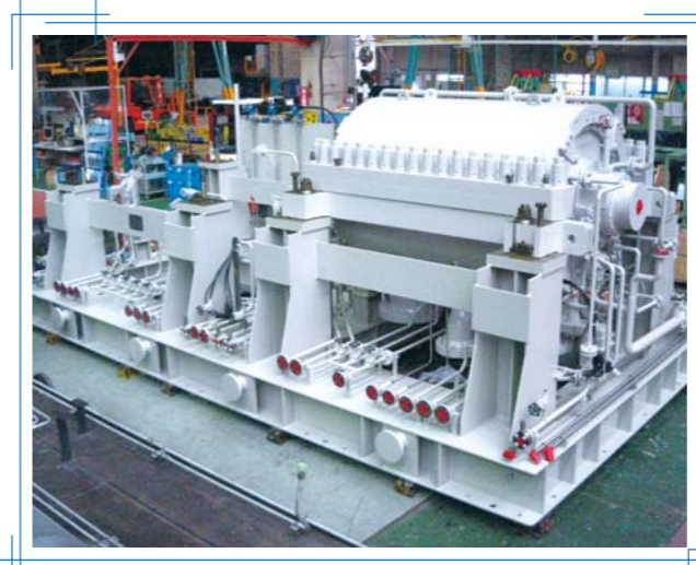
2MCH608 End Flash Gas Compressor
