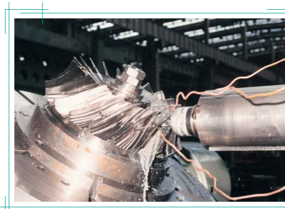
Five-Axis Machining of a Mixed Flow Impeller
