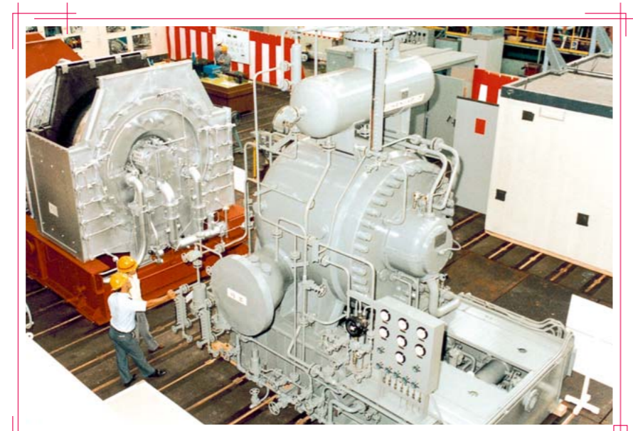
PCH802 Pipeline Booster Compressor
